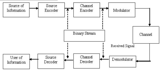
Fig 1.: Block Diagram of a Digital Communication System
