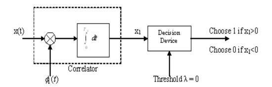
Fig (b) Coherent binary PSK receiver
