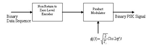
Fig(a) Block diagram of BPSK transmitter
