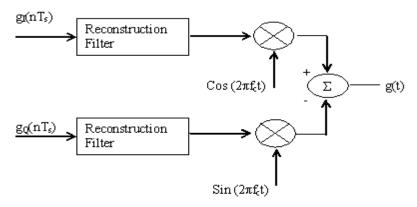
Fig: Reconstruction of Band-pass signal g(t)
